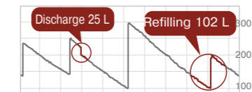
Change of the fuel volume in tank
