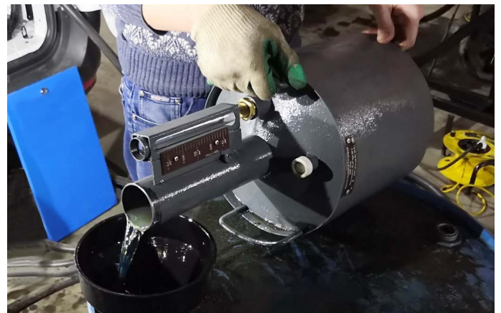
Manual calibration of the fuel tank using a measuring container takes several hours
