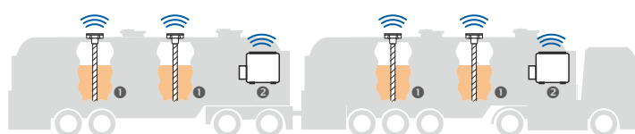
Monitoring system components: ① DUT-E 2Bio S7 fuel level sensors ② Teltonika telematics device with Bluetooth interface
